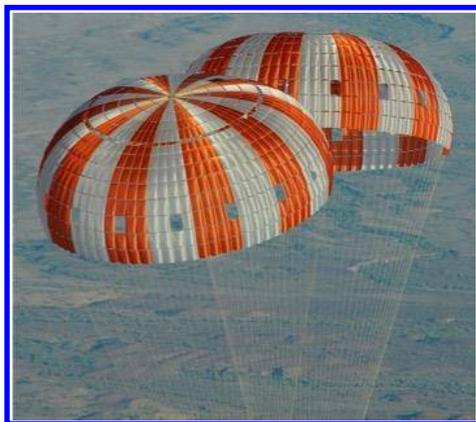
Figure 15. CDT-2-2 modified porosity.
