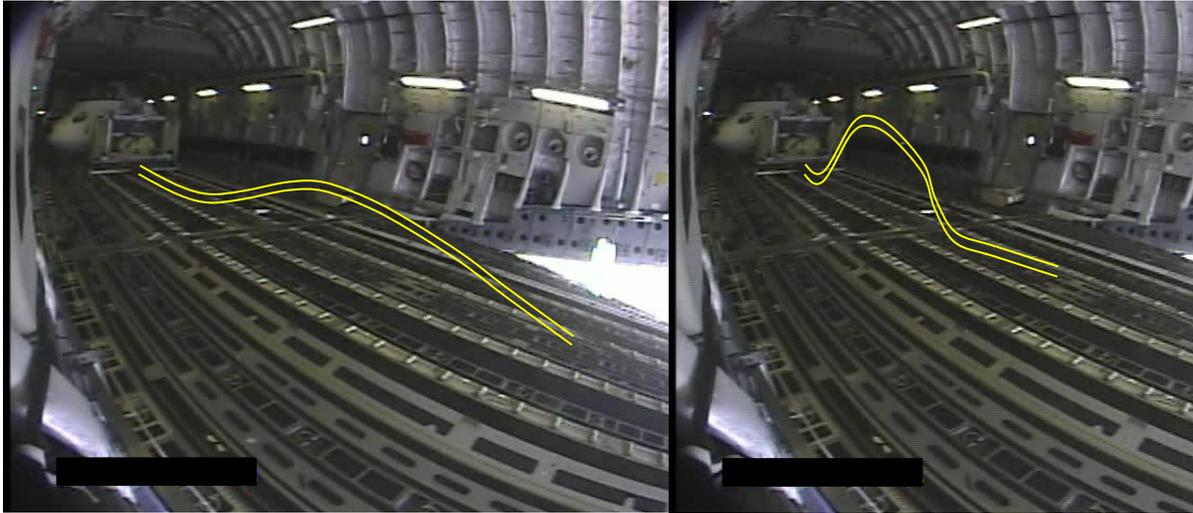
Figure 24. Extraction line “whip” effect on CDT-3-11.
