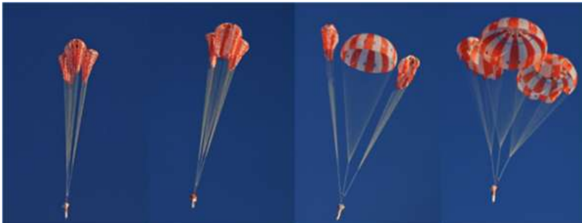
Figure 10. Progression of a Main parachute skipping second stage during CDT-3-4.
