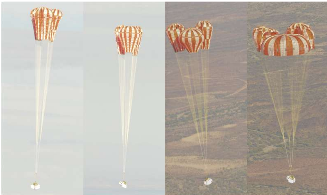
Figure 13. Progression of a Main skipping first stage during CDT-3-5.
