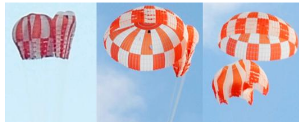
Figure 9. Main Parachute Unplanned Skipped Stage and Blanketing.
