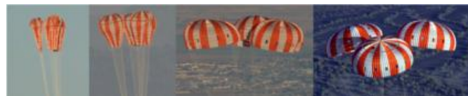
Figure 12. Main Parachute reefed stages.
