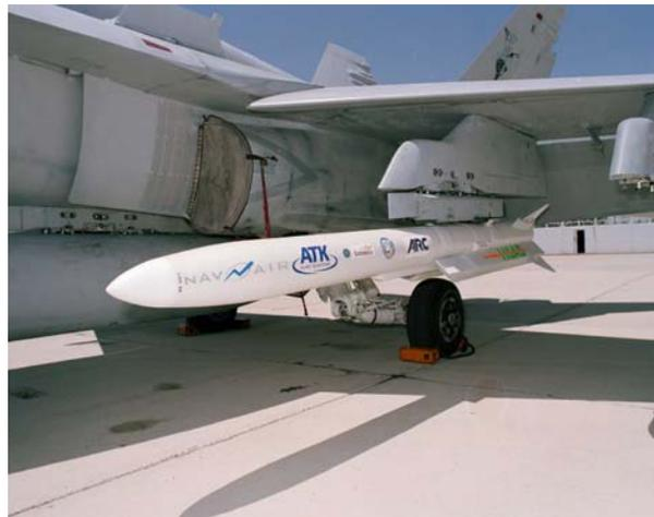
Figure 1. HSAD Missile on F/A-18C (baseline launcher).
